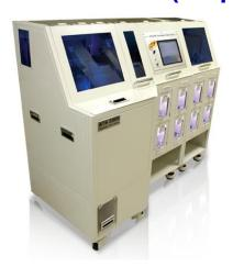
wise-ATS2000 is a tube sorting system that automates sorting process of pre-analysis and post-analysis and tube receiving in the diagnostic laboratory. It performs high-speed processing (more than 2,000 srots per hour) and tubes are grouped based on barcode recognition and the LIS tube information
