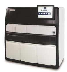
LIAISON® XL is a fully automated chemiluminescence analyzer, performing complete sample processing (sample pre-dilutions, sample and reagent dispensing, incubations, wash processes, etc.) as well as measurement and evaluation.
