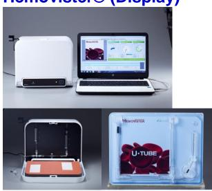
Hemovister® is an in-vitro medical device that measures both whole blood viscosity and plasma viscosity using patient's whole blood sample of 3ml.
